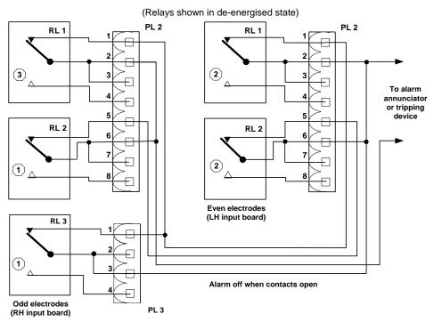
(Switch SW5 is set to EW for low-level alarms and set to ES for high-level alarms)
